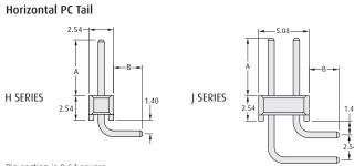
Pin section is 0.64 square. PCB mounting hole is Ø1.00 mm
