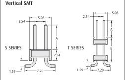
Pin section is 0.64 square. For PCB pad layout see page 131. S style only. B dimension is "0"
