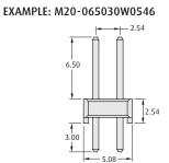
2.54mm Pitch vertical double row pin header with 5 pins per row and A dimension is 6.5 and B dimension is 3.0 in tin finish.
